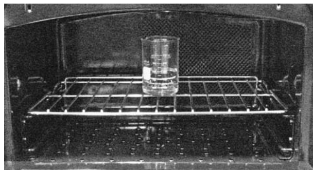
Figure 5.3: Water Load Placement
